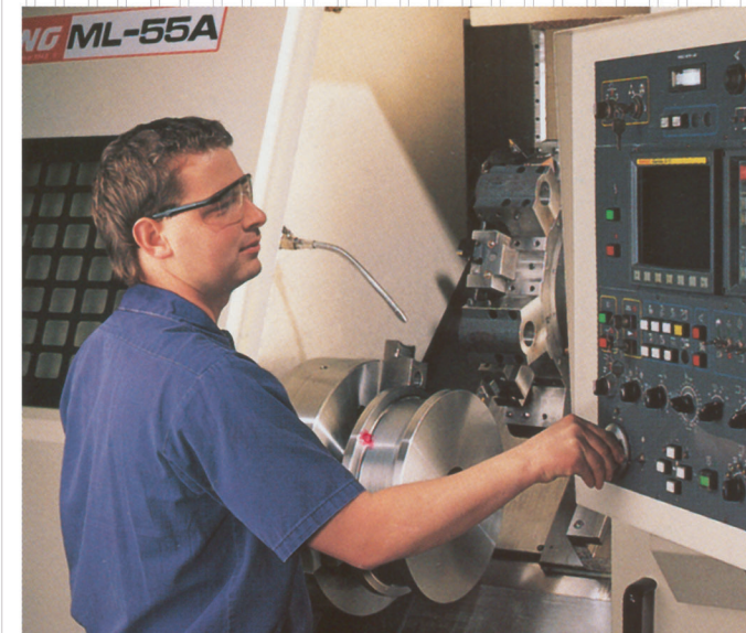
A machinist uses a CNC lathe to manufacture drums, wheels, axles and sheaves.
