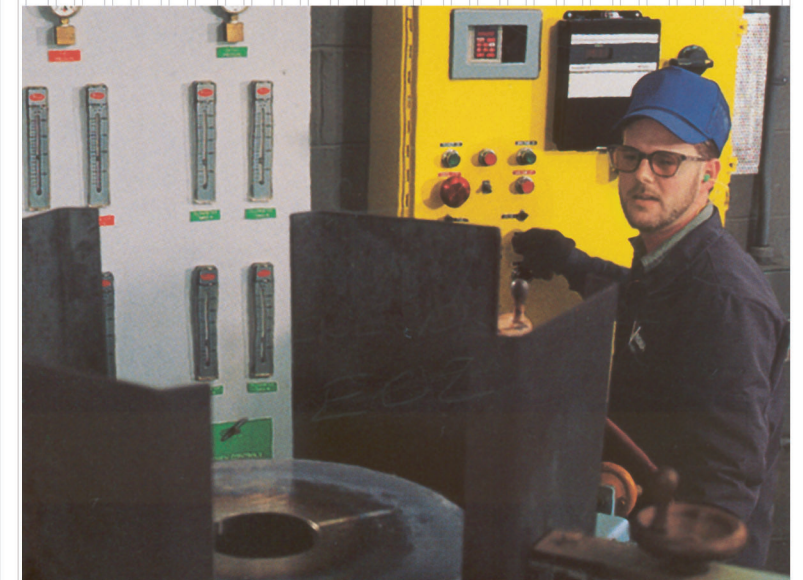
In-house flame hardening capability for wheels, sheaves and drums.
